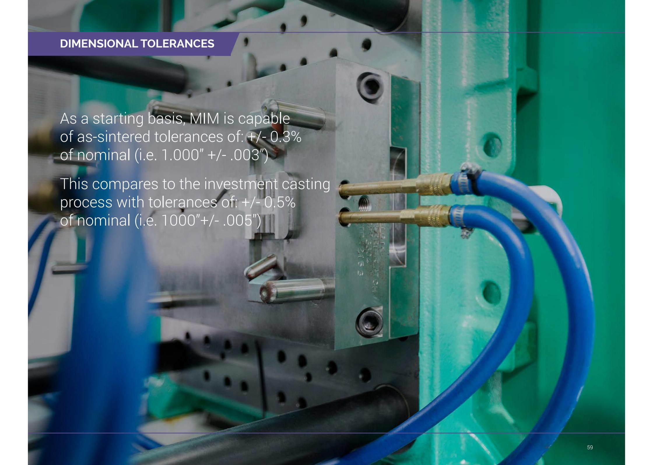
As a starting basis, MIM is capable of as-sintered tolerances of:  $\pm 0.3\%$  of nominal (i.e.  $1.000'' \pm .003''$ )
